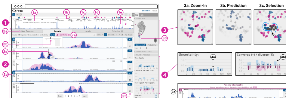
Figure 5: User Interface. The interface of PEAX consists of four main views: the (1) query, (2) list, (3) embedding, and (4) progress view. The pan-&-zoomable query view visualizes the data as blue bars that can superimpose the CAE's reconstruction as pink bars on demand (2). Besides optional metadata tracks (1a), PEAX draws region-based annotations at the top to indicate the prediction probability (1b), manual labels (1c), and custom window selections (1d). The list view (2) shows windows of sequential data for comparison and labeling. Aside is the embedding view (3) that shows windows as dots projected into a 2D canvas. By default blue dots stand for positive labels, pink stands for negative labels, gray represents no label, and black indicates the query. The progress view (4) visualizes metrics about the iteratively trained classifier as composed bar charts (4) where the dark (4a) and light (4b) bars indicate the progress in terms of the labeled and all windows respectively.
