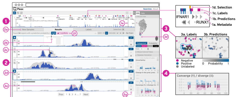
Figure 5: User Interface. The sequential data is visualized as blue bar charts (1&2), which can be superimposed with the CAE’s reconstruction as gray bars (2e). Additionally, the query view (1) can show metadata (1a-d) as region-based annotations. The list view (2) shows windows for comparison and labeling. The embedding view (3) represents windows as dots on a 2D canvas. The progress view (4) visualizes training metrics of the classifiers as composed bar charts (4), where the dark and light bars are relative to the labeled and all windows respectively.
