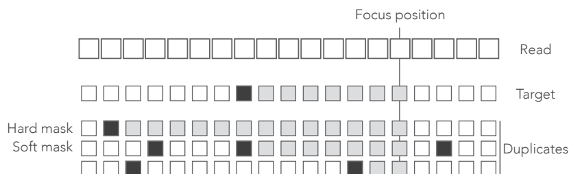
Figure 12: Example of hard and soft masks. Genomic sequences are shown below a read where open squares represent nucleotides. In the sequences, the open squares represent matches and the closed squares represent mismatches. The nucleotides contributing to the match length are represented as grey boxes. At the focus position, the match length of the target is 7. The first duplicate is a hard mask because its match length is 13 > 7 . The second duplicate is a soft mask because its match length is 7, as the target. The third duplicate is not a mask because its match length is 2 < 7 .
