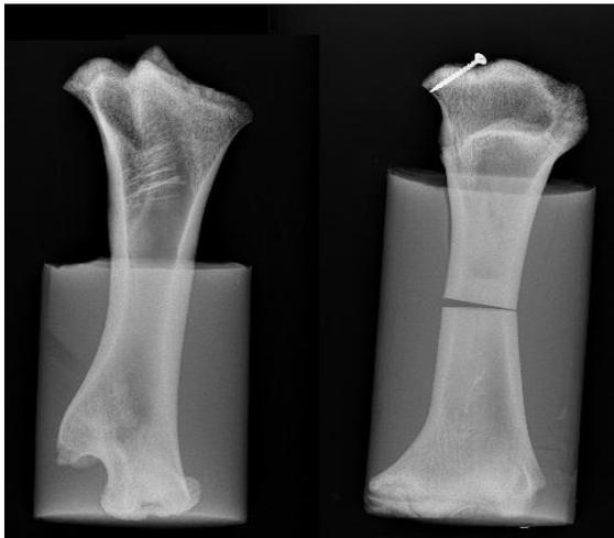
Fig. 2 Internal image of both phantoms: on the right radiography is evident the sharp fracture produced by a thin hacksaw. Both femurs show similar height and width.
