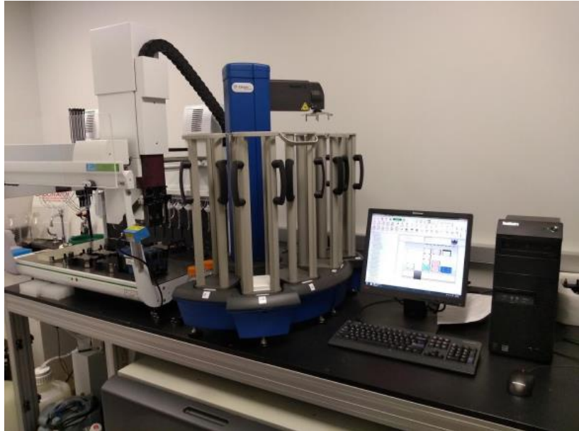
Figure 1. Centrifuge-free RABiT-II system for preparation of samples with automated liquid-handling system JANUS (PerkinElmer) and universal microplate handler Twister3 (Caliper Life Sciences).
