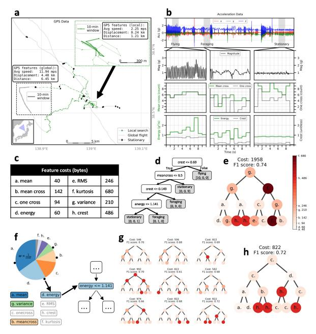
402 Figure 2. Creating AI models for sensor control onboard biologging devices. (a) Example GPS data
