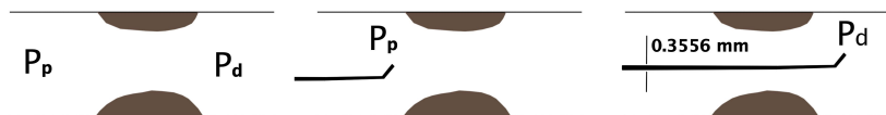
Fig 1. Left: The proximal ( P_p ) and distal pressures ( P_d ) near the stenosis. Middle: A flow wire measuring P_p before the stenosis. Right: A flow wire measuring P_d after the stenosis. The diameter of the flow wire is 0.014 inch (Volcano FloWire Doppler Guide Wire [3]).
