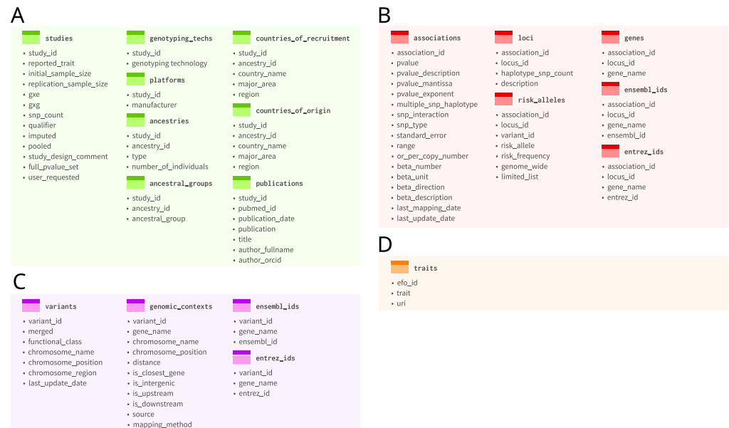
Figure 2. S4 representation of studies , associations , variants and traits . (A) S4 studies object, comprising 8 slots, i.e., 8 tables: studies , genotyping_techs , platforms , ancestries , ancestral_groups , countries_of_recruitment , countries_of_origin and publications . All tables share the primary key study_id . (B) S4 associations object, comprising 6 slots, i.e., 6 tables: associations , loci , risk.alleles , genes , ensembl_ids and entrez_ids . All tables share the primary key association_id . (C) S4 variants object, comprising 4 slots, i.e., 4 tables: variants , genomic_contexts , ensembl_ids and entrez_ids . All tables share the primary key variant_id . (D) S4 traits object, with one slot, i.e., one single tables: traits . The traits has the primary key efo_id .
