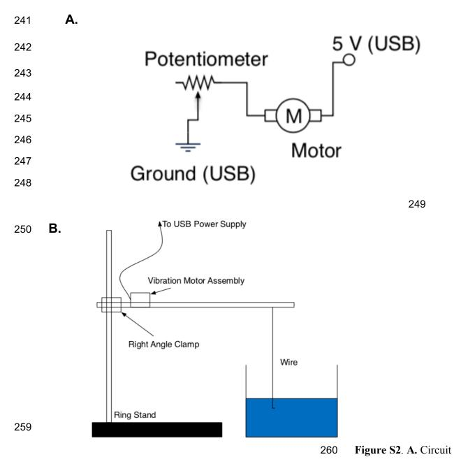
diagram of the excitation mechanism connected to the plastic rods. **B.** Set-up for the VAB trials.
