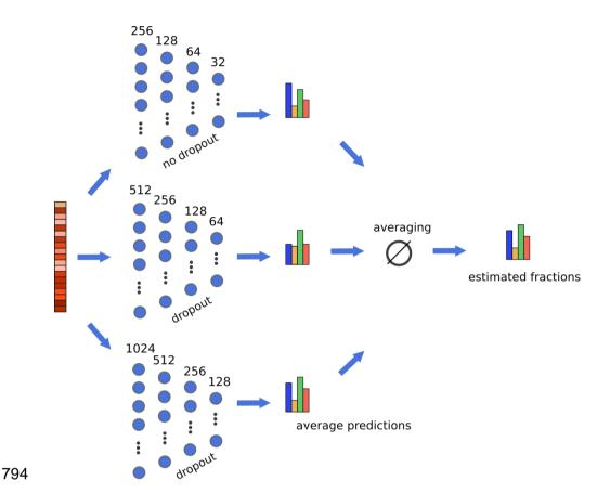
Figure S1 Overview of the Scaden neural network ensemble model. A bulk RNA-seq sample is the input to three separate deep neural networks with varying layer sizes and dropout regularization. The predictions of all three models are subsequently averaged to obtain the final Scaden predictions. During training, predictions are not averaged and each model is trained separately.
