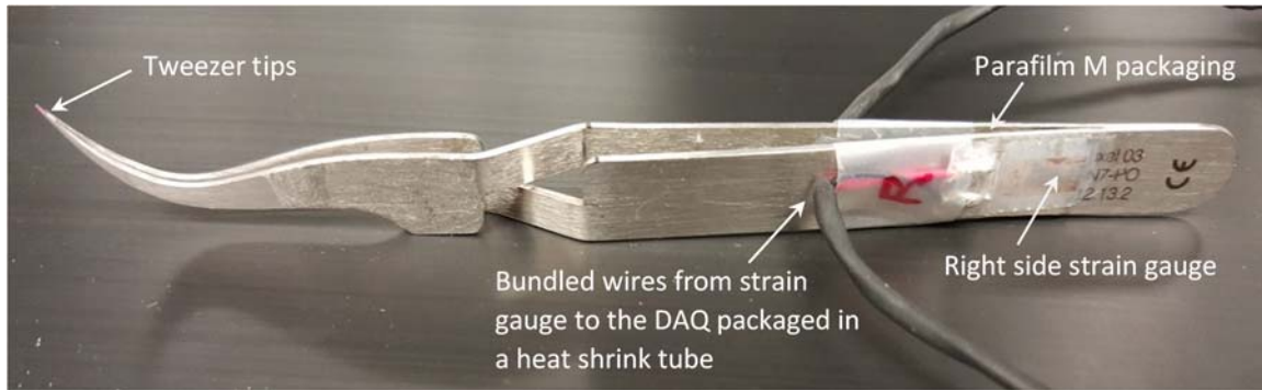
Figure 1. Cross-action Dumont #N7 tweezers instrumented with miniature precision foil strain gauges and packaged to protect against damage due to mechanical handling.
