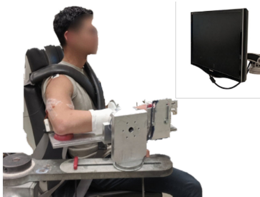
Figure 1: Isometric joint torque recording device with high-density surface EMG grids on the biceps brachii and triceps brachii.
