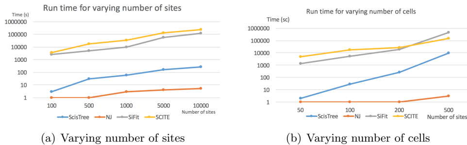
Figure 6: Average running time (in seconds) for a single simulated dataset of ScisTree, neighbor joining (NJ), SiFit and SCITE. Time for increasing the number of sites m (with 100 cells) is in part 6(a), and the time for increasing the number of cells n (with m being five times of n ) is in part 6(b).
