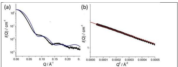
**Figure 2.** (a) SAXS profiles for OLDNs. Black dots show the experimental SAXS profile, and a blue line indicates the calculated profile based on the crystal structure (PDB: 5GSE). (b) Guinier plots. Filled circles are the experimental results, and the red line shows the result of the least square fitting with the Guinier formula (see text).
