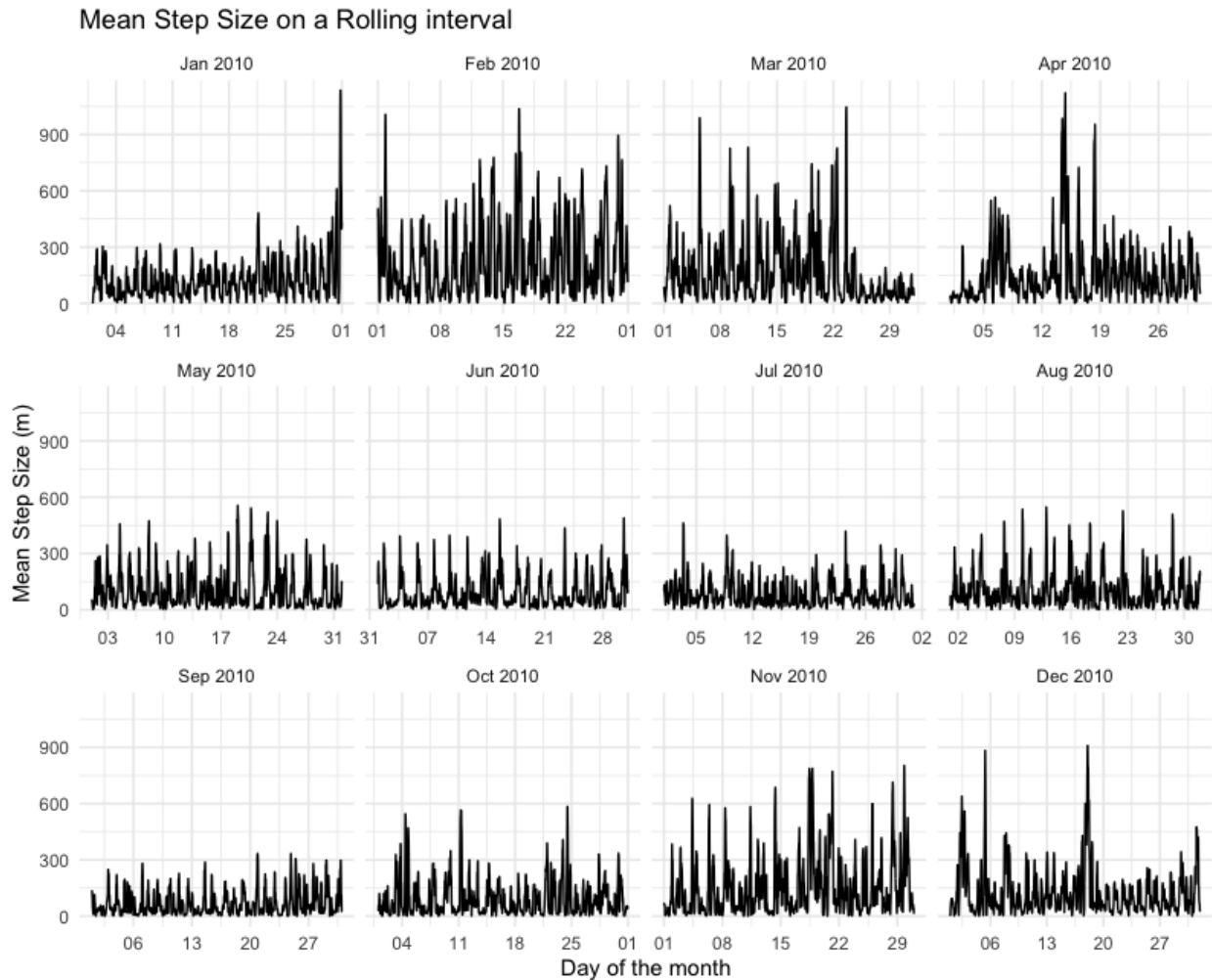
Figure 6: Rolling Step Size. A faceted plot of step size averaged using a rolling window of 3 hours using stmove 's rolling_stats function. stmove reports include plots of rolling means for step length ( s_t ) and turning angle ( \theta_t ), as well as rolling autocorrelations of both ( s_{t-1}s_t and \theta_{t-1}\theta_t ) and a rolling cross-correlation between them ( s_t\theta_t )
