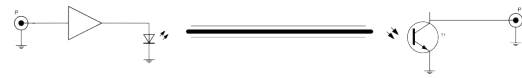
Fig. 3 Optical communication scheme. A TTL signal comes out of a digital Arduino port is amplified and converted into light through a LED. The light is transmitted through an optical fiber to the terminal where it will be converted into a TTL signal.
