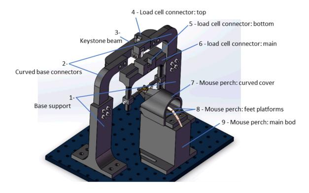
Instructions for assembling the head fixation apparatus:
