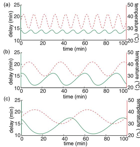
**Figure 2.3. Amplitude of the delay changes with the period of the time-varying temperature.** Time-varying delays (green solid lines) corresponding to various time-varying temperature  $T(t) = \Delta T \sin(\omega t) + T_0$  (red dashed lines). Parameter values here are  $\theta = 4500K$ ,  $E = 13.5 \text{ min.}$ ,  $\Delta T = 6^\circ C$ ,  $T_0 = 36^\circ C$ , and  $\delta_p = .28$ . (a)  $\omega = \frac{2\pi}{10}$ . (b)  $\omega = \frac{2\pi}{30}$ . (c)  $\omega = \frac{2\pi}{50}$ .
