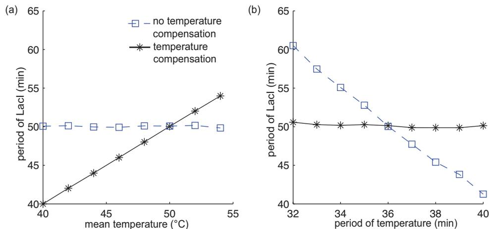
**Figure 3.2. Entrainment of the synthetic gene oscillator with and without a temperature sensitive promoter.** (a) Period of the circuit with and without temperature compensation for  $\omega = 2\pi/50 \text{ min}^{-1}$ ,  $\Delta T = 2^\circ C$ , and different mean temperatures  $T_0$  in Eq. (2.12). (b) Frequency entrainment of the circuit with and without temperature compensation for  $\Delta T = 2^\circ C$  and  $T_0 = 36^\circ C$ .
