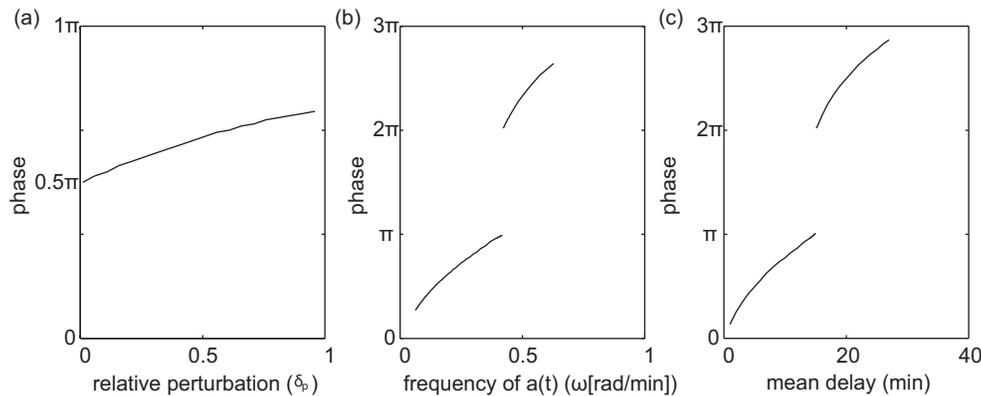
**Figure 2.5.** Phase shift between  $a(t)$  and  $\tau_{\text{eff}}(t)$  as a function of  $\delta_p$ ,  $E$ , and  $\omega$ . (a) phase shift as a function of  $\delta_p$  with  $E = 15$  and  $\omega = 2\pi/30$ . (b) phase shift as a function of  $\omega$  with  $E = 15$ , and  $\delta_p = .5$ . (c) phase shift as a function of  $E$  with  $\omega = 2\pi/50$ , and  $\delta_p = .5$ .
