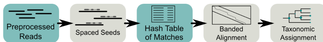
Figure 1 – Schematic overview of MALT. For each preprocessed metagenomic sequencing read, the algorithm generates all contained spaced seeds and looks them up in a hash table of spaced seeds representing the reference database. A banded alignment is calculated for each match of seeds. Once all alignments for a given read have been calculated taxonomic binning of the read is performed using the LCA algorithm.
