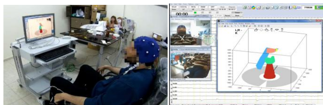
Fig. 7. Online experiments in which the participants have controlled a 3 dof-robot manipulator arm using EEG BCI.
