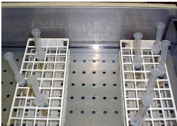
**Figure 2. Simulation of vibrational forces encountered in spaceflight.** A shaking water bath simulates the vibrational accelerations to which the bacteria would be exposed in the spaceflight environment. In microgravity, vibration may be the major accelerational force acting upon the organisms. The 10-mL syringes approximate the Fluids Processing Apparatus (BioServe Space Technologies, Boulder, CO), the “test tubes” of biological experiments performed in space.
