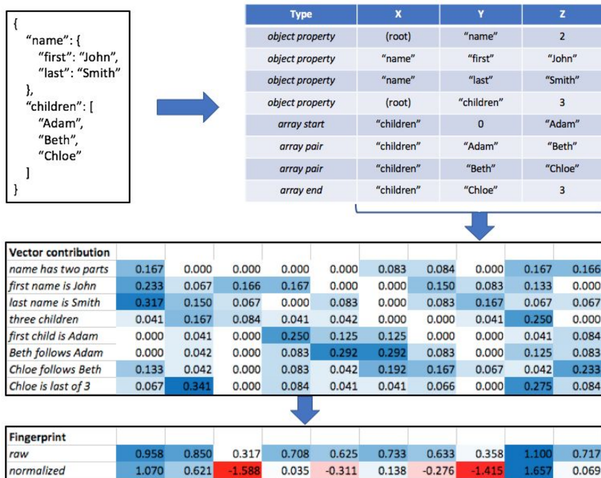
Figure 1. Overview of the strategy. Semi-structured data (here shown as a JSON object, upper left) is transformed into a series of statements (upper right) describing local substructure within objects and arrays. Each statement is then independently encoded into a numerical vector (in the example at the center, of length 10) as described in the Methods. The sum of these vector contributions (bottom) yields the 'raw' fingerprint, which can then be centered and rescaled to yield the 'normalized' fingerprint.
