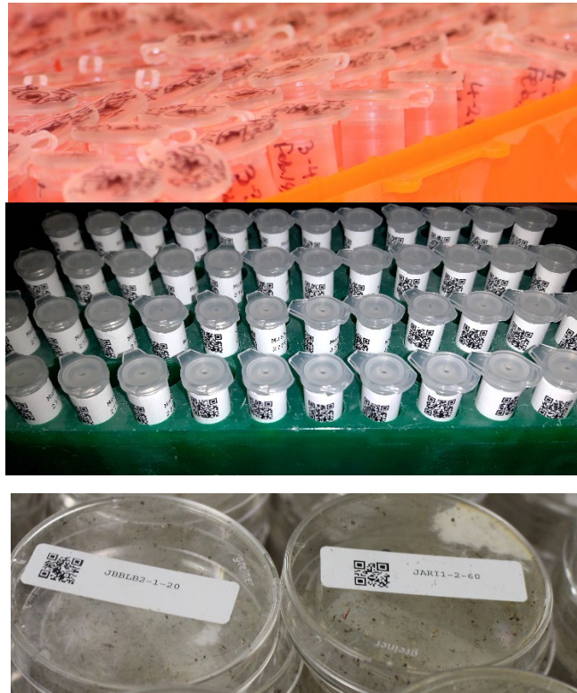
Figure 1. Examples of conventional, hand-labelled tubes (top panel), compared with tubes (mid panel) and petri dishes (lower panel) labelled with digital barcodes and human-readable text labels created using the baRcodeR package.
