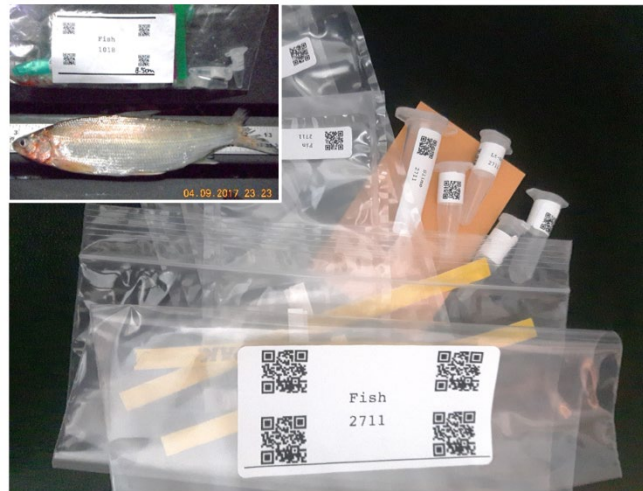
Figure 4. Sampling kit demonstrating the use of baRcodeR to improve data integrity and repeatability of sampling methods. A sample bag for each fish is shipped to the field; each bag contains labelled containers for various tissue subsamples. In this example, separate labels were created with baRcodeR to encode the same fish ID #2711 into the bag containing the fish, as well as all subsamples associated with it. Inset shows a cropped archival picture of fish #1018, which visually links a fish ID code to its collection date and time, fish length and species ID.
