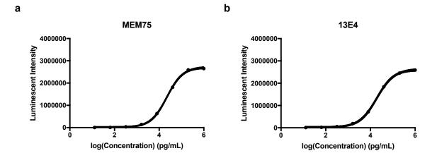
Standard curves for the binding of (a) MEM75 and (b) 13E4 antibodies to iPS-BMVECs that were used in the ELISA experiment.
