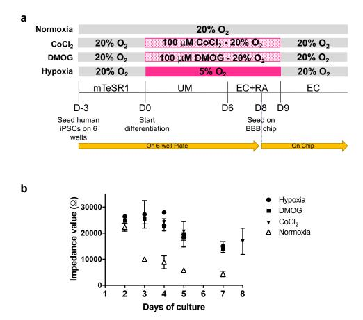
(a) Experimental design schematic showing how BBB Chips were generated using iPS-BMVECs differentiated under normoxia (as control), hypoxia, or using chemical inducers (CoCl<sub>2</sub> and DMOG) that mimic hypoxia under normoxic conditions. (b)
