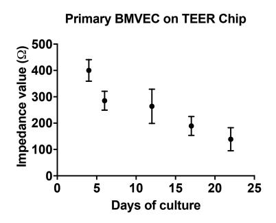
Barrier integrity of the primary human BBB Chip monitored in TEER chips with impedance measurements, recorded in the frequency range of 0.1 Hz to 100 kHz over 3 weeks after seeding primary BMVECs along with astrocytes and pericytes.
