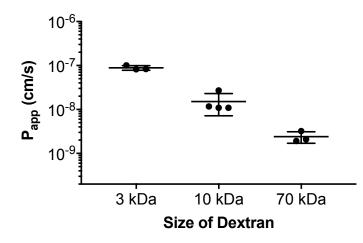
Permeability of dextran tracers of various sizes in the BBB Chips. Fluorophore-labelled dextran molecules (3, 10, or 70 kDa) were flowed through the brain channel on the BBB Chips for 3 h at 100  $\mu$ L/h flow rate. Effluent samples from both brain and vascular channels were collected and fluorescent intensity of the samples were detected, and dextran concentrations were quantified based on standard curves to calculate P<sub>app</sub> values.
