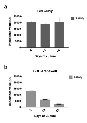
The high barrier function (impedance measured by TEER) was sustained for longer times in BBB Chips with iPS-BMVECs that were induced to differentiate using CoCl<sub>2</sub> interfaced with astrocytes and pericytes(**a**) and this effect appeared to require flow as it was not observed when the same cells were interfaced in static Transwell cultures (**b**). Barrier integrity on the BBB Transwells was monitored by TEER measurements.
