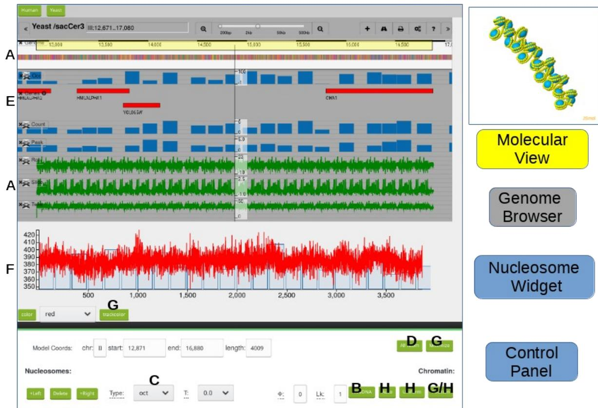
**Figure 3: Summary of G-Dash Views:** G-Dash contains an embedded genome browser (Biodalliance), a Nucleosome Widget, a Control Panel, and a Molecular Viewer (JSmol). The Nucleosome Widget is a component of the Control Panel that displays a Nucleosome Energy Landscape and allows nucleosomes to be individually manipulated. See text for additional descriptions of Control Panel elements. Letters corresponds to descriptions in text and items in Figure 4.
