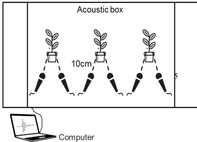
**Figure 1. Experimental setup.** In each recording, three plants are placed inside an acoustic box with two directional microphones oriented at each plant. Using two microphones helps eliminating false detections resulting from electrical noise clicks of the recording system and cross-
