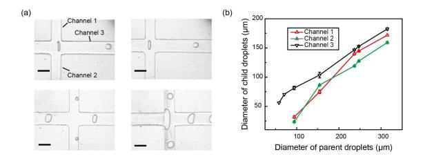
Figure S2. The effect of mother droplet size on the resultant daughter droplets in oneto-three junctions. (a) The amount of daughter droplets increased from one to three, as the size of mother droplets increased. Scale bar, 200  $\mu$ m. (b) The diameters of daughter droplets plotted as a function of the diameter of mother droplets. Channel names are designated in Figure S2a.
