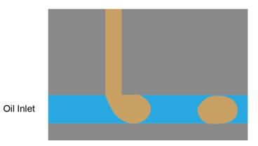
Figure S1. Generation of mother droplets using T-junctions.
