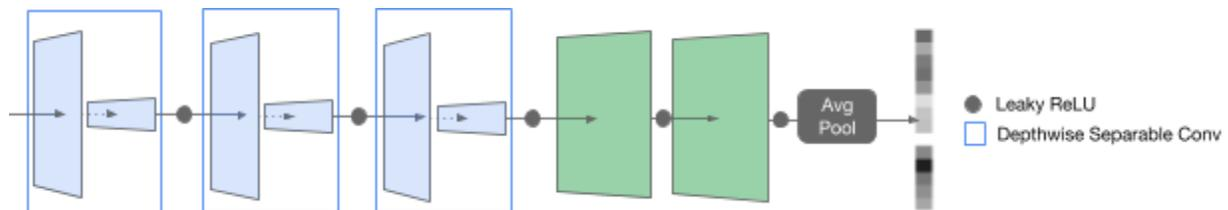
**Figure 1: Overview of the proposed neural network architecture.** The neural network architecture used in this study consists of three depthwise separable convolutional filters followed by two or three fully-connected layers (in green), which are tiled as needed along the length of the input and combined via an average pooling layer prior to the softmax output layer.
