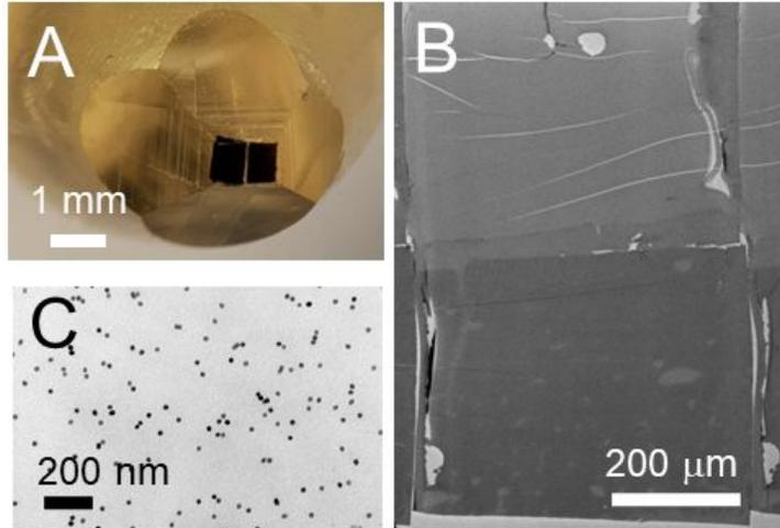
**Figure 1. Magnetically augmented resin.** A) View of a magnetically augmented resin block, showing the parts containing superparamagnetic particles (black, left) and biological tissue (black, right). B) Electron transmission image of an ultrathin section, showing the tissue resin at the bottom and the magnetic resin at the top. C) Close-up EM image of the magnetic resin, showing superparamagnetic nanoparticles of circular shape.
