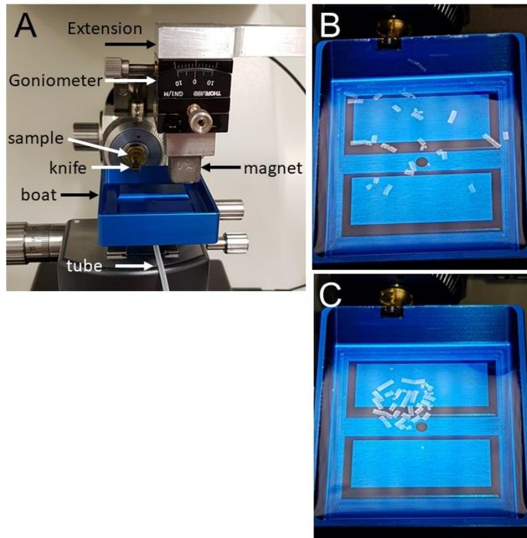
**Figure 2. Magnetic section collection (MagC).** A) MagC setup. B) Free-floating magnetically augmented sections (gray) are dispersed on the water surface. C) After scanning the magnet across the sections 1 mm above the water surface, the sections are concentrated near the center of the boat.
