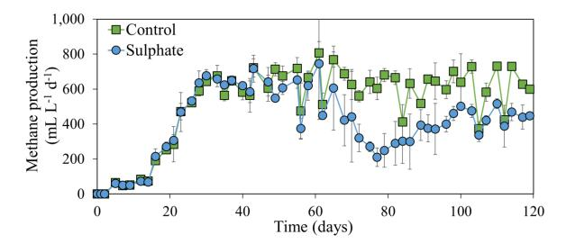
**Figure 1** Methane production in function of time in the Control and Sulphate digester. Average values of the biological replicates (n=3) are presented, and the error bars represent standard deviations.
