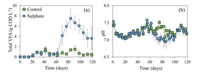
**Figure 2** Total volatile fatty acid (VFA) concentration (a) and pH (b) in function of time in the Control and Sulphate digester. Average values of the biological replicates (n=3) are presented, and the error bars represent standard deviations.
