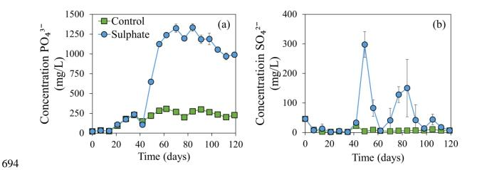
**Figure 3** Phosphate (a) and sulphate (b) concentration in function of time in the Control and Sulphate digester. Average values of the biological replicates (n=3) are presented, and the error bars represent standard deviations.
