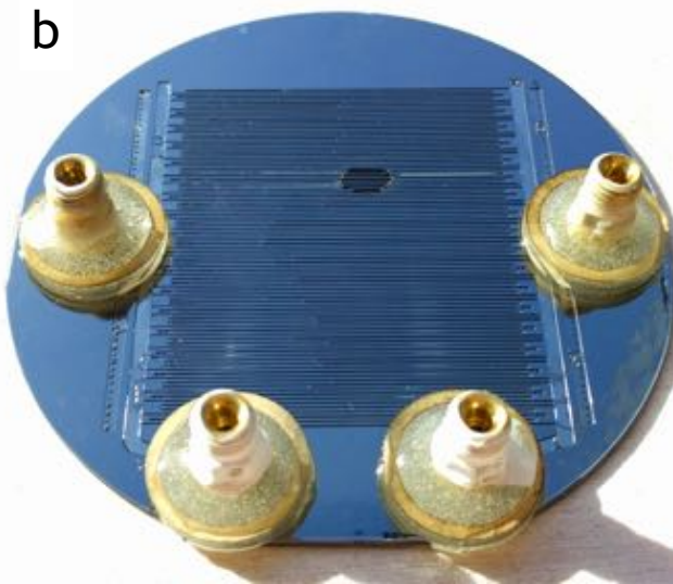
Figure S11: a. 20k-VLSDI chip leaking while operating at low flow rates due to debris and weak anodic bonding between glass and silicon. b-c. Optical images show broken position of the 20k-VLSDI chip while operating at low flow rates as shown in a.
