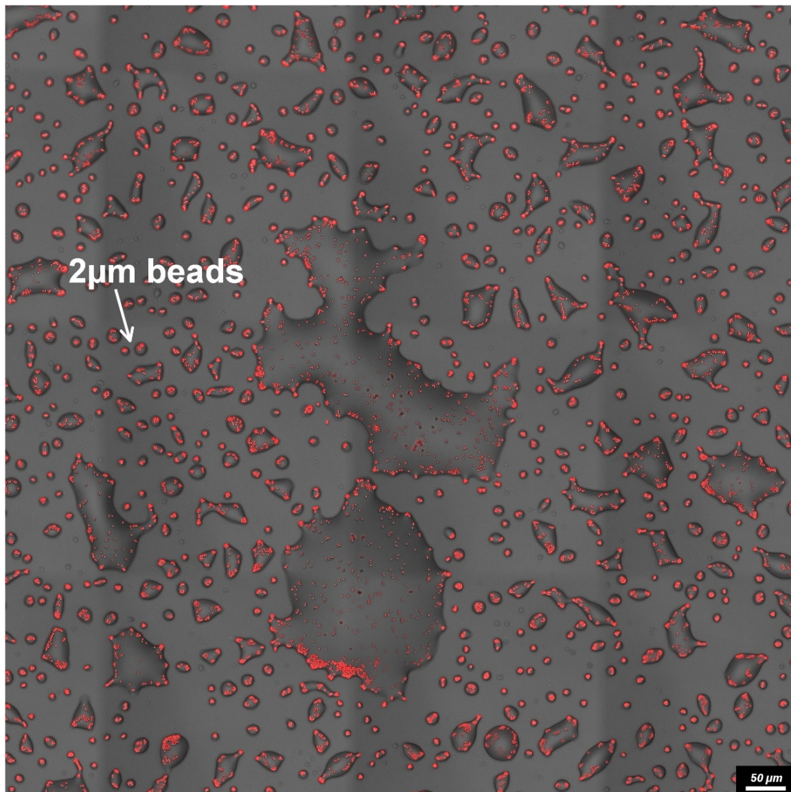
Fig. S1. Microscopic wetness – experiment with fluorescent beads (2µm diameter). Experiment was performed under same conditions as the experiments with bacteria (M9 diluted x2, 28°C, 85% RH; see Methods).
