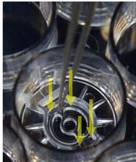
Figure 1: Load device into well plate. Ensure device is flat by pushing down in multiple places (indicated by yellow arrows).
