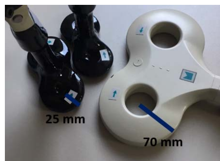
Figure 1. Comparing the Magstim “25mm coils” (left) to a Magstim 70mm coil. TMS with the two “25mm coils” was applied in a shifted fashion to reduce inter-coil-distance.
