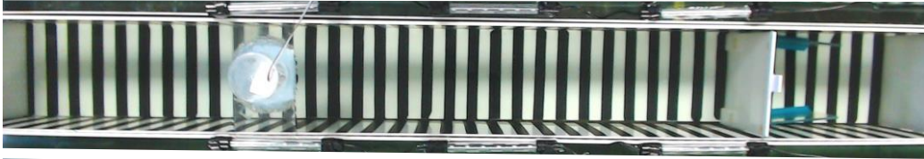
Figure 1: Overhead photo of main set-up in position +10. Two perforated white screens either end ensure laminar flow and prevent the fish from seeing outside of the tank. The start area is 30cm long, and the overhead infrared detector sits overhead 80cm from the start area doorway. This in turn controls aquarium lights running along the top of the maze walls symmetrically on either side.
