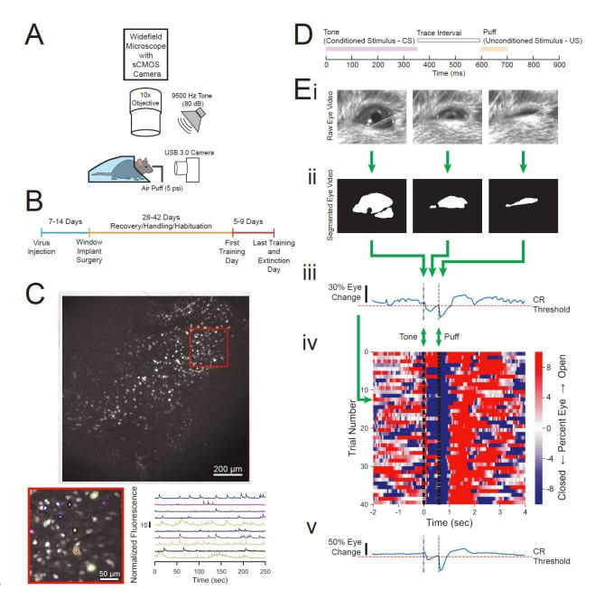
**Figure 1. Experimental design and measurement of animal behavior. (A)** Imaging and behavioral setup. The imaging setup consisted of a microscope with a sCMOS camera, standard wide-field fluorescence optics, and a 10x long working distance objective to image a head-fixed mouse. For the behavioral paradigm, a speaker was positioned near the mouse and a cannula for directing an air puff was placed in front of the right eye. Eye responses were monitored using a USB 3.0 Camera. See methods for
