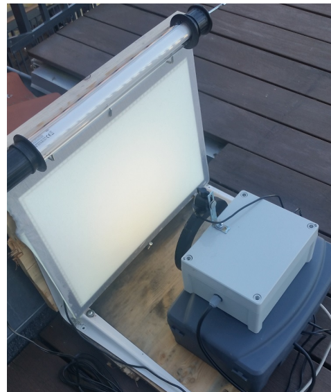
Figure 4: Photo of the light trap and computer vision system.
