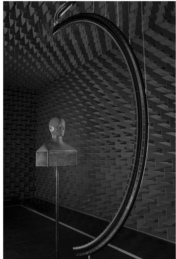
Figure 1: The HRTF Arc with 64 loudspeakers, exemplarily an artificial head is positioned in the center [2].
