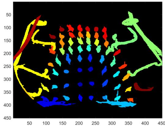
**Fig. 11.** Final segmentation of the electropalatogram. Wires and electrodes are labelled with different colours for visualisation purposes. It should be noticed that there are some minor artifacts, which may be removed with further post-processing.
