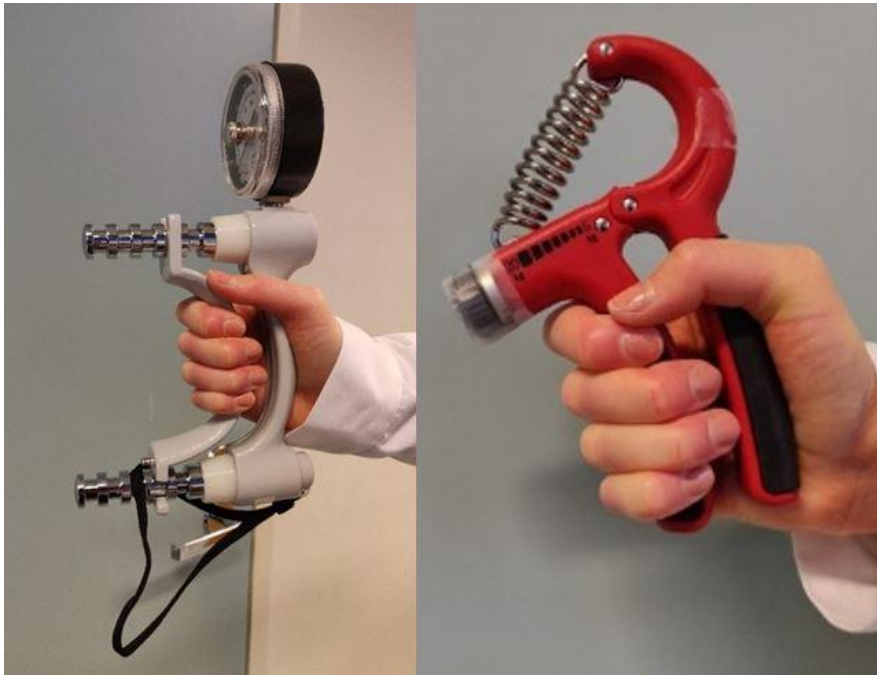
Figure 1. Hand grip strength measurement device (left) and hand grip endurance task device (right)
