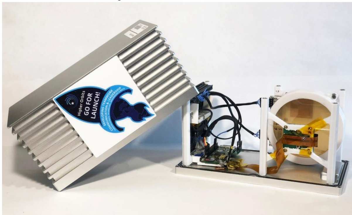
Figure S1: Fabricated flight hardware unit, packaged in a 2U Space Tango CubeLab™. Media Courtesy: Space Tango, Inc.
