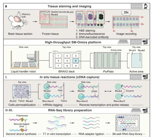
BRAVO deck: 1-trash, 2-tips full box, 3-robot arm, 4-thermo block 4°C-65°C, 5-Ø, 6-thermo block 4°C-65°C, 7-magnet, 8-tips empty box, 9-Ø
