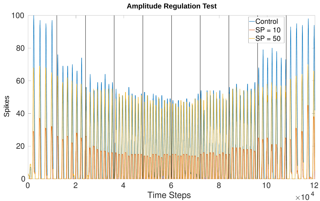
Figure 11: Comparison of amplitude when running the network unregulated versus creating a set point (SP) at 10 spikes and 50 spikes. The SP in this plot is equivalent to the "desired spike value" referred to in Equation (6). There is more overshoot for lower frequencies as compared to higher frequencies but the change in amplitude is visible from the control experiment where w_{max} is applied uniformly. Vertical lines indicate when a change in voltage threshold potential occurs thereby changing the frequency. The threshold updates every 1,200 time steps (1.2s) creating a total of 10 divisions. V_{th} starts at -54.81mV producing a frequency of 3.77Hz and increases to -50.79mV producing a frequency of 9.14Hz . After 6,000 time steps V_{th} decreases again, returning to a value of -54.74mV producing a final frequency of 4.00Hz . The middle two trials from 4,800-7,200 time steps are held at the highest V_{th} , around -50.79mV . The values fluctuate by hundredths of a mV because V_{th} is affected by current noise.
