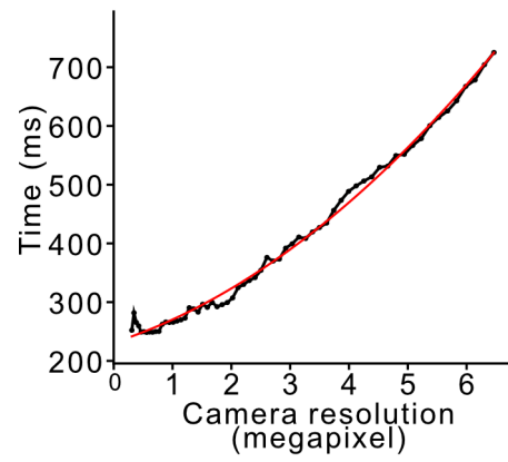
Supplementary Figure 3: Latency of closed-loop control applications. Latency of closed-loop control as a function of camera resolution. Red line shows a second order polynomial fit of y = 6.8x^2 + 32.6x + 231 .
