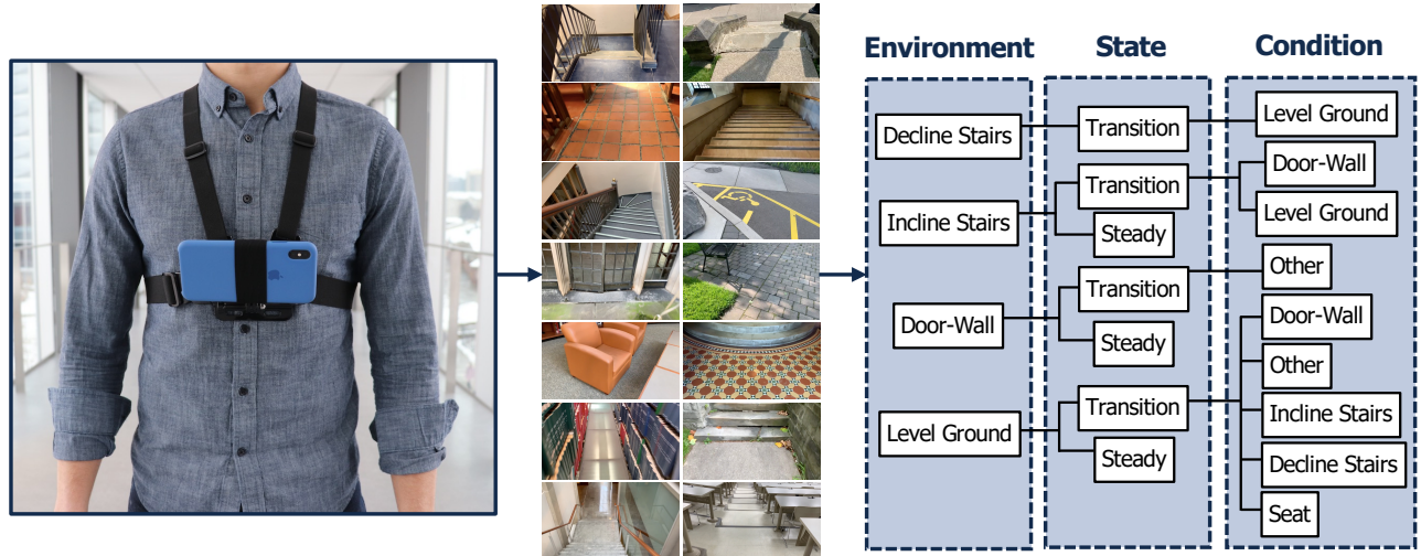
Fig. 2 Development of the ExoNet database, including (left) photograph of our wearable camera system used for large-scale data collection; (middle) examples of the high-resolution RGB images of walking environments; and (right) schematic of the 12-class hierarchical labelling architecture [11].
