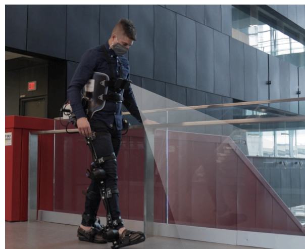
Fig. 1 Photograph of the lead author wearing our robotic exoskeleton with environment sensing superimposed.
