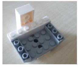
We call this the objective, because it is really like a microscope objective. By the way, the lens comes from the camera of an old iPhone 5.
