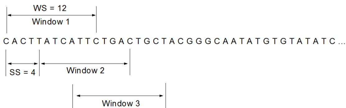
Figure 2. Example of computing the Information Entropy Spectrum of a genome by sliding a window across it, with window size is WS = 12 and step size is SS = 4 .
