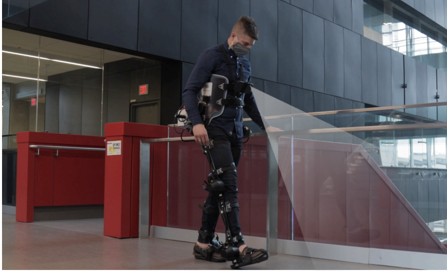
Figure 3. Photograph of the lead author walking with our robotic exoskeleton with camera-based environment sensing superimposed.
