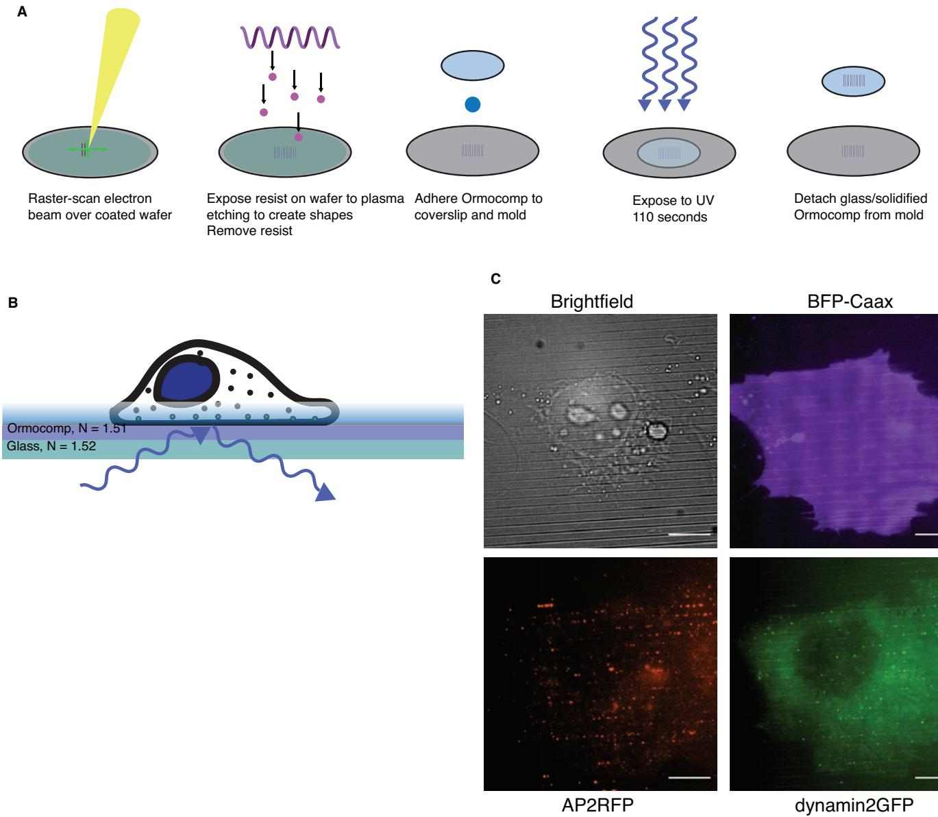
**Fig. S1. UV-Nanoimprint Lithography creates glass-like substrates for induced curvature studies.** (A) Method of silicon mold production and Ormocomp substrate manufacturing. (B) Ormocomp's refractive index allows for TIRF microscopy of live cells. (C) TIRF microscopy of a cell grown on 120-nanometer ridges expressing BFP-Caax, AP2RFP, and dynamin2GFP simultaneously.
