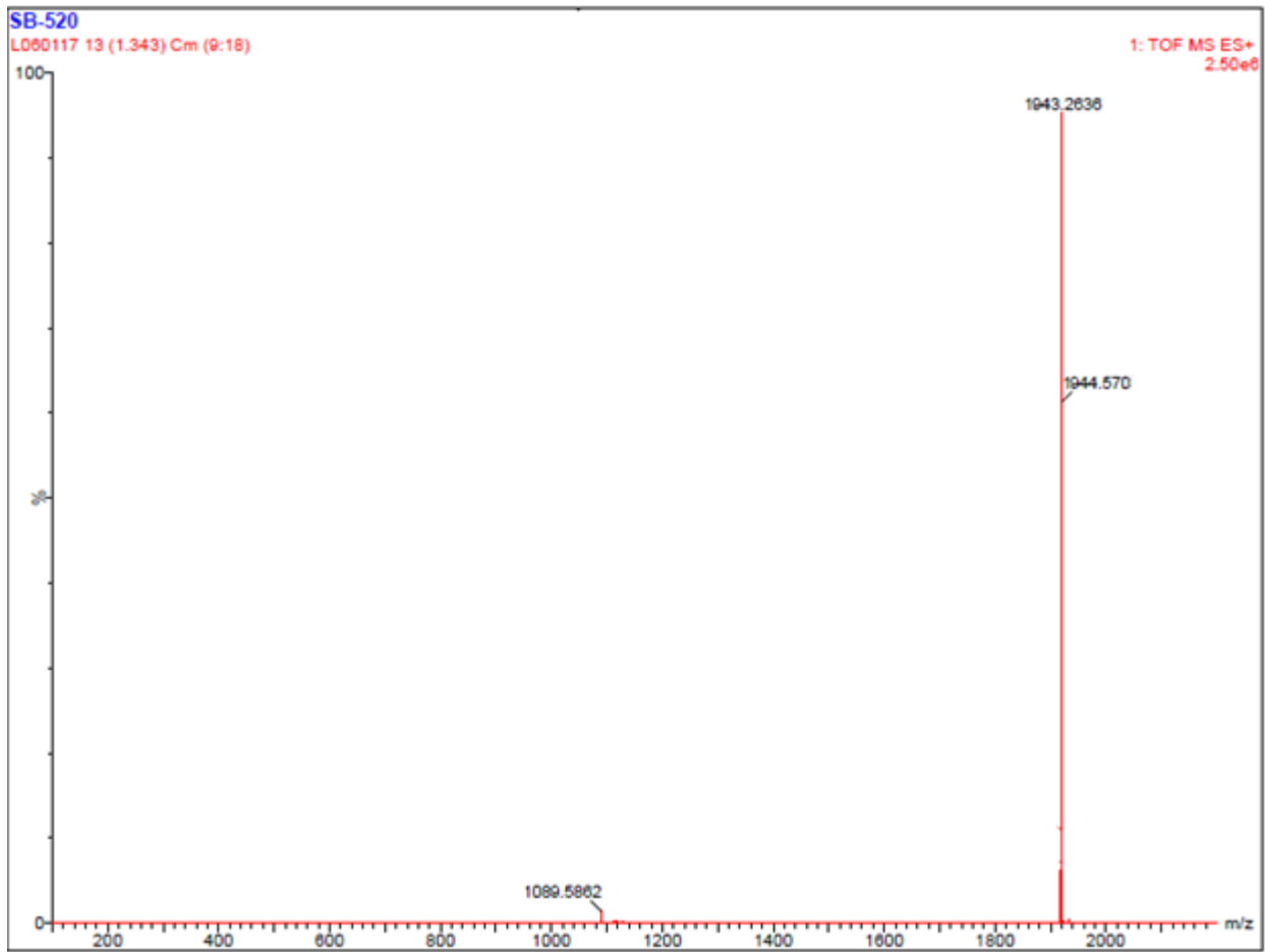
Figure S9: Section of HRMS (ESI): m/z [M + Na]^+ spectra for the synthesized peptide 27 . calcd for C_{98}H_{157}N_{19}O_{20}Na : 1943.1750; found: 1943.2187.
