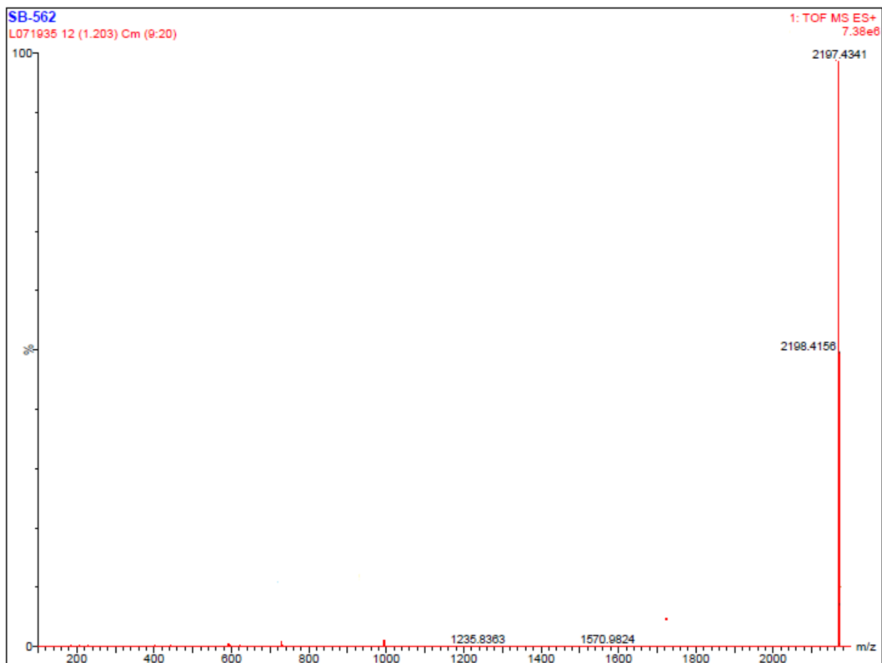
Figure S2: Section of HRMS (ESI): m/z [M + Na]^+ spectra for the synthesized peptide 20 . calcd for C_{112}H_{187}N_{23}O_{20}Na : 2197.4221; found: 2197.4341.
